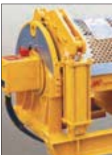
⇄ Drum brake with skid frame on LS2000R
